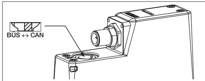
Fig. 15: Switch for setting the fieldbus, type 8742.
