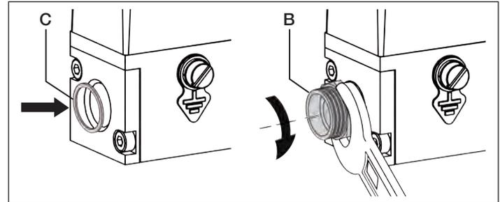
Fig. 10: Fix the sealing ring and screw on the connecting thread
