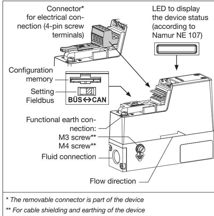
Fig. 1: Design of the device type 8741
