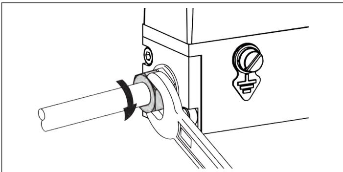
Fig. 12: Tighten the union nut.
