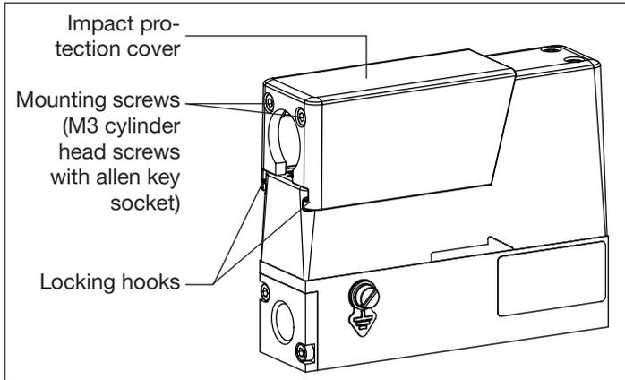
Fig. 13: Attaching the impact protection cover
