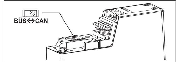
Fig. 14: Switch for setting the fieldbus, type 8741.
