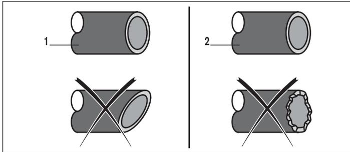
Fig. 8: Cutting the pipe and deburring
