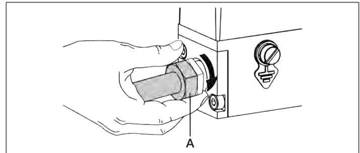
Fig. 11: Insert pipe and tighten the union nut.
