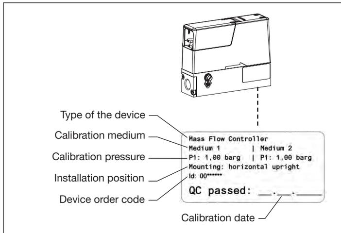
Fig. 5: Location and description of the calibration plate
