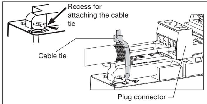
Fig. 18: Attached cable with strain relieved by cable ties
