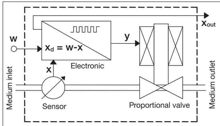
Fig. 3: Function diagram of the MFC (Mass Flow Controller)
