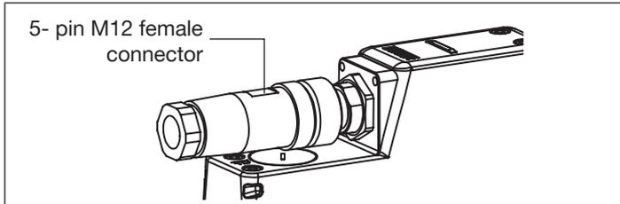
Fig. 20: Screwing in the M12 female connector
