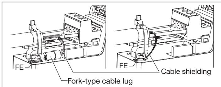
Fig. 22: Cable shielding connection
