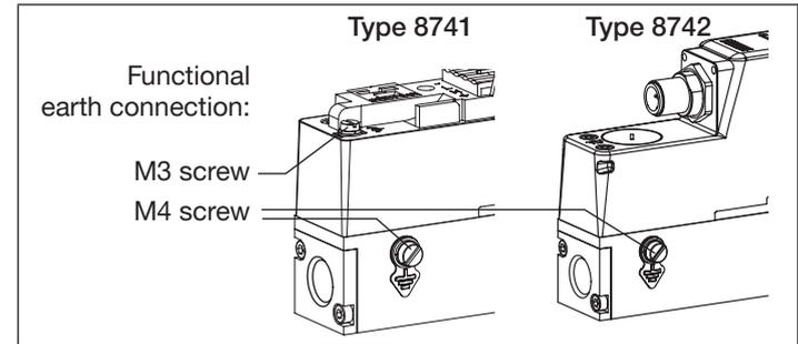
Fig. 21: Connection options for functional earthing FE
