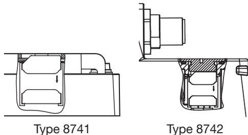
Fig. 24: Replacing the configuration memory
