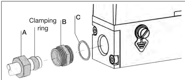
Fig. 9: Slide the union nut and clamping ring onto the pipe.
