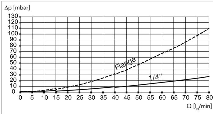
Fig. 4: Pressure loss diagram, for air, with a 250 µm input filter, for an MFM
